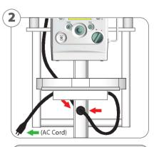
Once Power Supply is secure in the Compartment pull the remaining length of the Power Supply Cord through the Opening located below tray on the Central Bracket. This will keep the Cord safely tucked behind the Ventilator and Rolling Stand.
