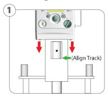
Loosen black knob on rear of rolling stand track to back screw out of track. Slide Ventilator down into track, making sure Ventilator's track is vertically aligned with the Rolling Stand's track.
