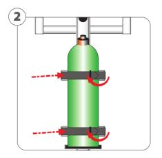
Once cylinder is stable slip velcro straps through D-rings to secure the cylinder. Give Cylinder a tug to test resistance.
