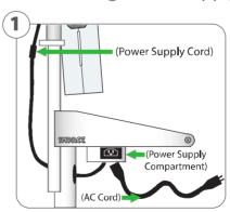
Insert Power Supply into the Compartment located directly underneath the tray. Feed Power Suppy Cord through the opening in the rolling stand, connect cord into ventilator. Lastly Connect AC Cord to Power Supply Compartment and insert into an AC Outlet.
