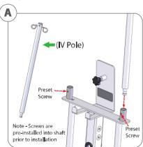
Using the 5/32" Hex Wrench and preset screw (5/16-24 x 1/4") insert the IV pole to a preferred side and tighten until IV pole is secure. Removal of IV Pole should not be possible if connected properly.
