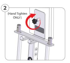
Once Ventilator is secure in track, turn the black knob clockwise to secure Ventilator in place. To release Ventilator turn the knob counter clockwise, loosening the Ventilator from track and slide up vertically.
