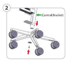
Once wheels are connected and locked, align Central Bracket to the center of Base. Insert bottom of bracket into opening located in the center of base. Using the 5/16" Hex Wrench screw the 1" Button Head Screw along with the 2" Flat Washer provided, creating a secure connection.
