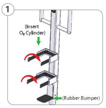
Insert Oxygen Cylinder between the brackets located on the rear of the Rolling Stand. Cylinder should be resting on the Rubber Bumper for proper installation.
