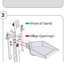
Align the tray's openings then using the 5/16" Hex Wrench screw each of the four 3/4" Flat Head Screws into each of the four openings on the Central Bracket. Screws should be secured tightly for user and patient protection.
