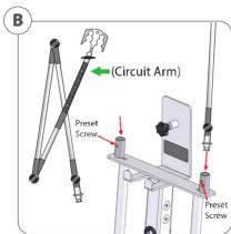
Using the 5/32" Hex Wrench and preset screw (5/16-24 x 1/4") insert the Circuit Arm to a preferred side and tighten until Arm's pole is secure. Removal of Circuit Arm should not be possible if connected properly.
