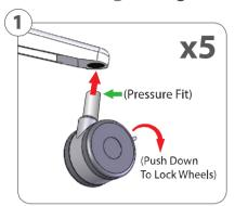
Lock each wheel prior to attaching to base, then Connect each of the 5 Locked Wheels to each of the coinciding openings at the bottom of Base. Each wheel shall connect easily when pressure is applied from opposite ends of base and wheel bottom.
